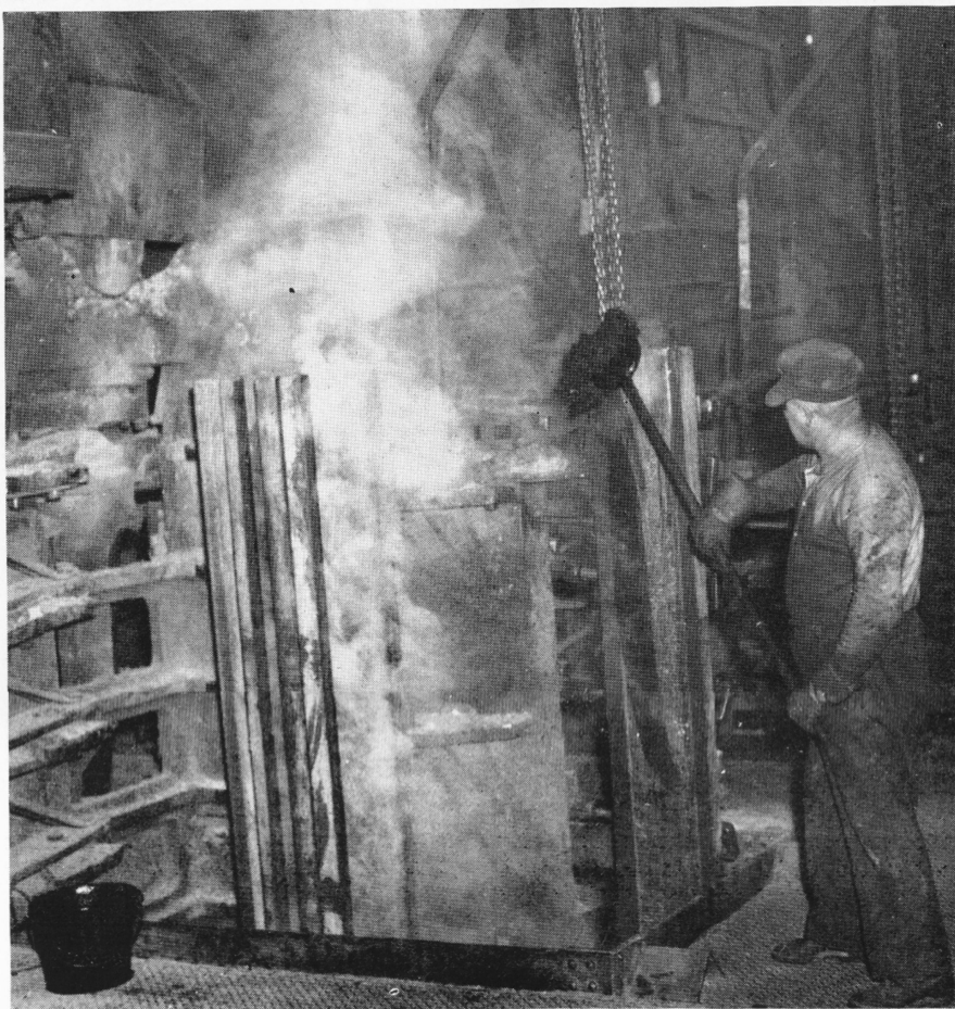
Typical of the way the Casting Shop is going out after better and better production records is this shot of Ted Kunco, a moldman at the Scovill Casting Shop. Ted is greasing the molds for another pour from the casting furnace before the molds are cold after the previous pour. Notice how the heat from the molds vaporizes the grease. That's production and it's growing!
